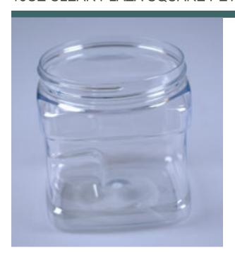
Size 16.00 OZ Overflow Capacity 603.00 cc Neck Diameter 89.00 Neck Finish 400 Material PET Color **CLEAR** Shape **SQUARE** Item Weight 39.50 g Item Height x Width/Diameter 3.7 in x 3.6 in Blow Technology **ISBM** PCR Possibility Yes
